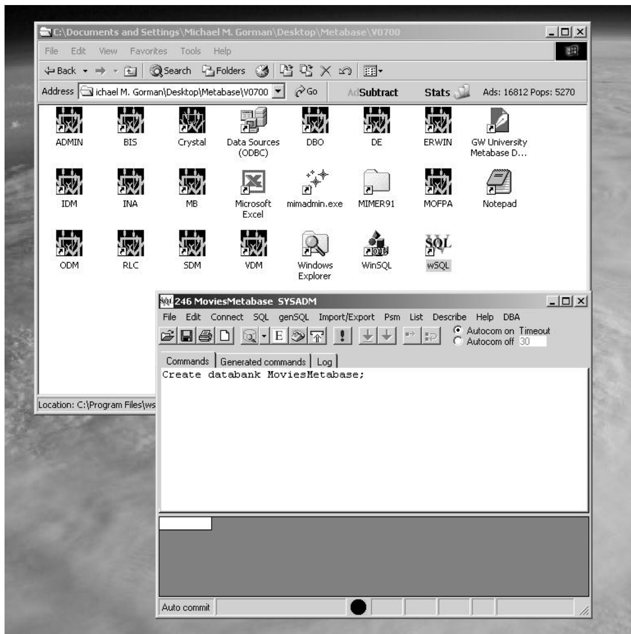
Figure 10. Entering the Create Databank Mimer command.
